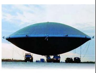
The "Locomoskayner" airship takes to the air with nothing more than helium, but will also have special outfitted hot air cells to regulate its buoyancy, RIA Novosti news agency reported.
